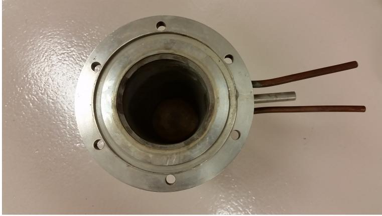
Fig. IV.5.: A picture of the refiner vessel's copper cooling jackets and vent.
