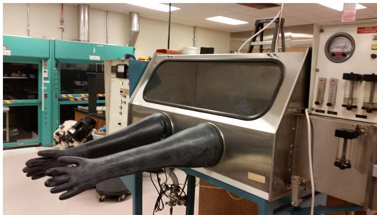
Fig. IV.1.: A picture of the glove box at the Fuel Cycle and Materials Laboratory, Texas A&M University.
